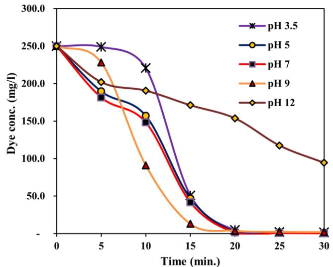
Fig. 5. Effect of initial pH on the final dye concentration: initial dye concentration = 250 mg/l, volume of solution = 1 liter, NaCl Concentration = 1 gm / l, applied voltage = 10 V
