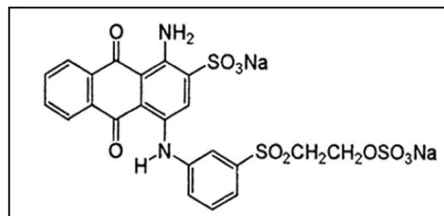
Fig. 2. Chemical structure of Reactive Blue 19
